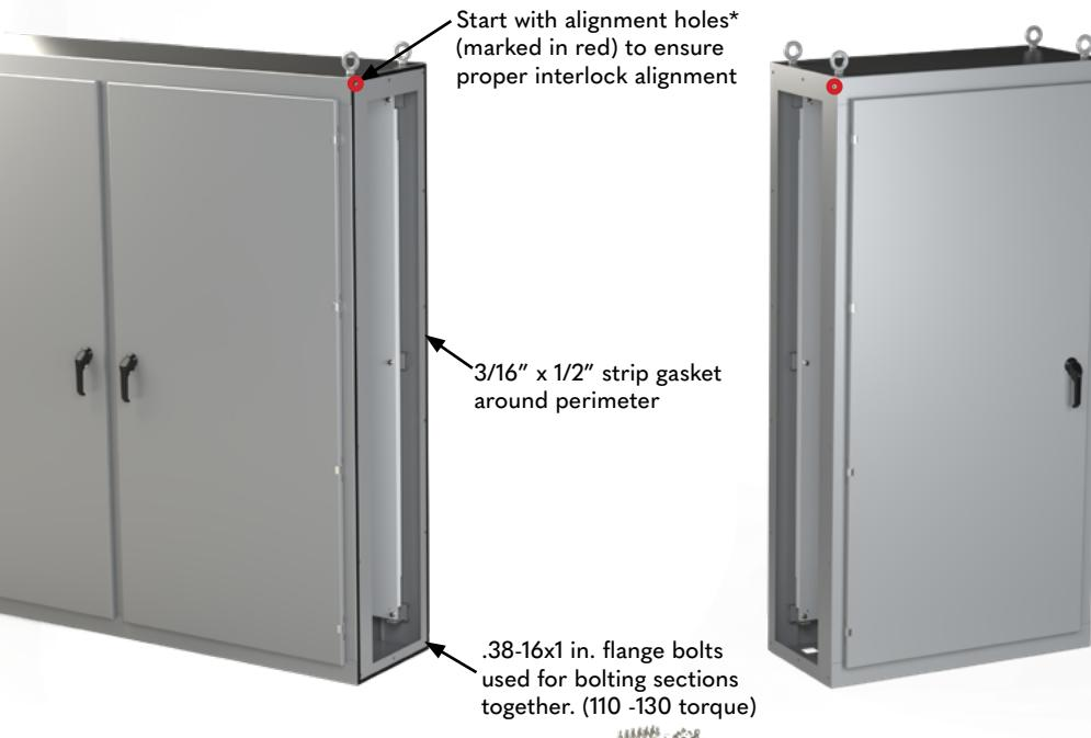
\*Two alignment obrounds are located on the front side of the enclosure. These are used for the [cable interlock](#).
