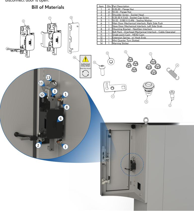
1. Install NEXD to main enclosure. (For installation and mounting hole pattern see <a href="nexd-install.pdf">nexd-install.pdf</a>)
