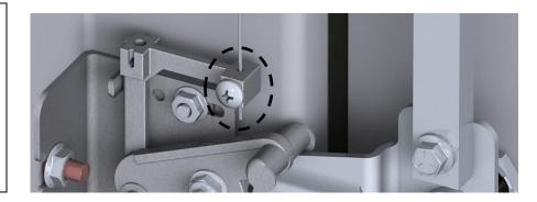
7. -CLOSE THE DOOR AND DOOR HANDLE FULLY AND THE OPERATING HANDLE SHOULD BE DEFEATED TO TURN THE DISCONNECT TO THE "ON" POSITION. VERIFY THEN THAT DOOR ENGAGES THE HOOK WHEN YOU TRY TO OPEN THE DOOR.
