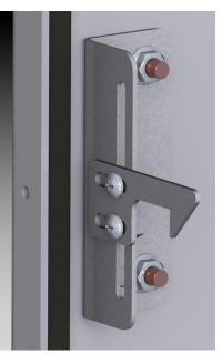
6. -NOW YOU CAN ADJUST THE MDV. WITH THE DISCONNECT OPERATING HANDLE STILL IN THE "OFF" POSITION SIMPLY PULL THE CABLE DRAWING DEFEATER STRIKE DOWN SO THAT THERE IS ABOUT A 3/8 INCH BETWEEN THE DEFEATER AND THE DEFEATER STRIKE AND TIGHTEN THE SCREW TO LOCK IN POSTION.
