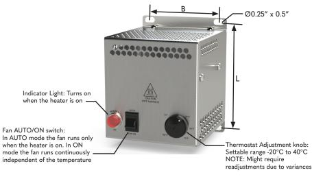
Additionally the heater element has an over-temperature thermostat that will turn off the heater when the outlet temperature becomes excessively high as a result of a fan failure or blocked airflow.
