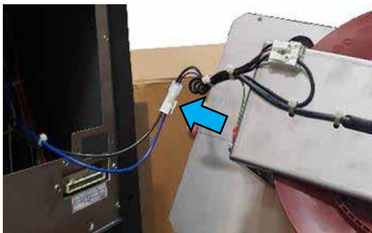
Step 19: Connect internal fan assembly power connector,
