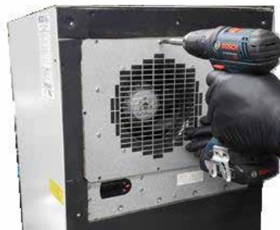
Step 20: Mount the internal fan assembly.
