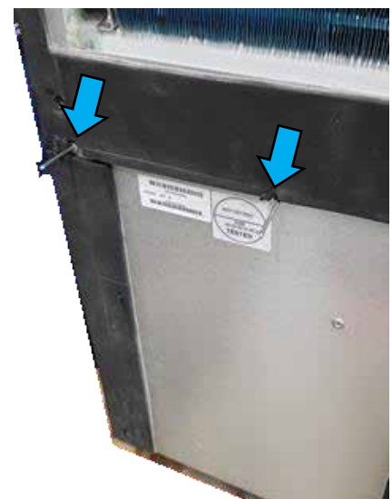
Step 15: Once new assembly is in place install eight rivets.
