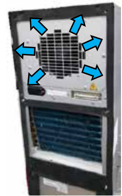
Step 27: Mount the internal fan assembly as shown
