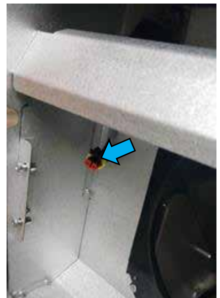
Step 10: When removing ambient fan assembly disconnect power connector.
